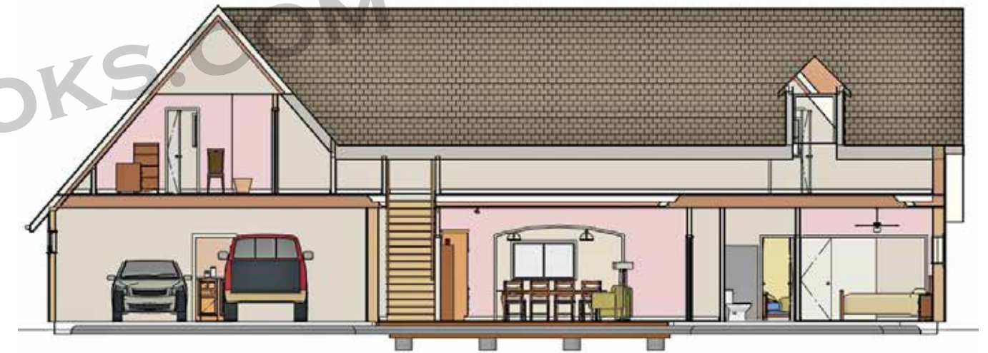
Figure 8-4. A “section” drawing that shows how furnishings and vehicles fit into the house.
