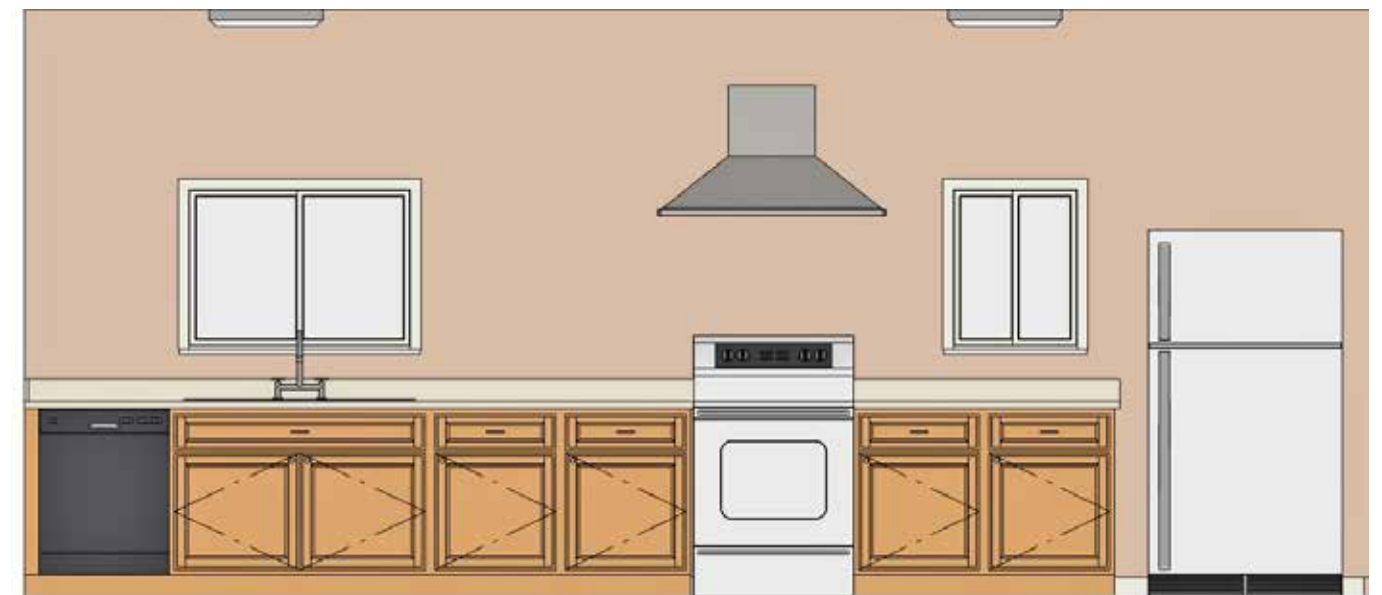
Figure 8-3. “Interior elevation” of a kitchen. It shows the locations of cabinets and appliances, and wall colors. The vee symbols on the cabinet doors are a standard method of indicating the sides where the hinges are installed.
