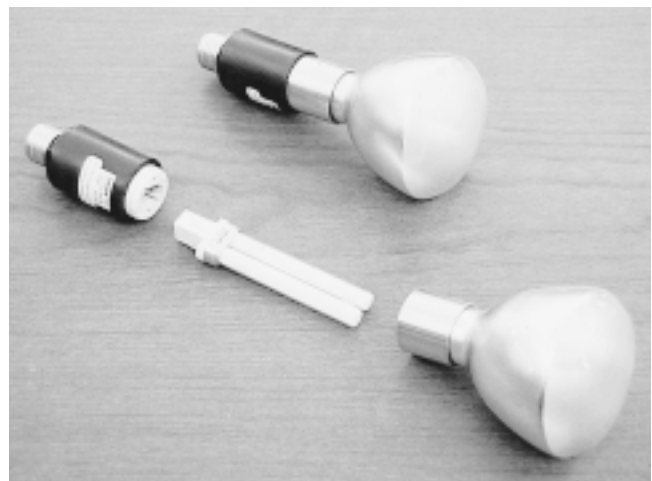
Fig. 4 Reflector fixture with separately replaceable lamp The ballast may last several times longer than the lamp. A unit like this should be made of glass, rather than plastic, because the ultraviolet radiation from a fluorescent lamp will darken plastic.
