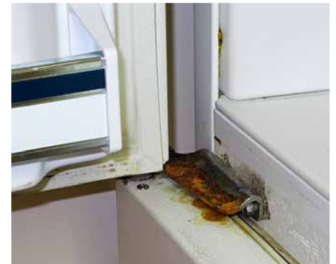
Figure 7-2. Rust that results from condensation around the opening of a refrigerator door.
