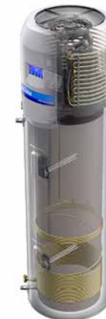
Figure 5-19. Heat pump water heater. The heat pump on top of the tank has coils that extract heat from the surrounding air. The heat is sent to coils in the bottom of the tank. This unit also has two electric resistance heating elements, which supplement the heat pump when the air temperature is too low.
