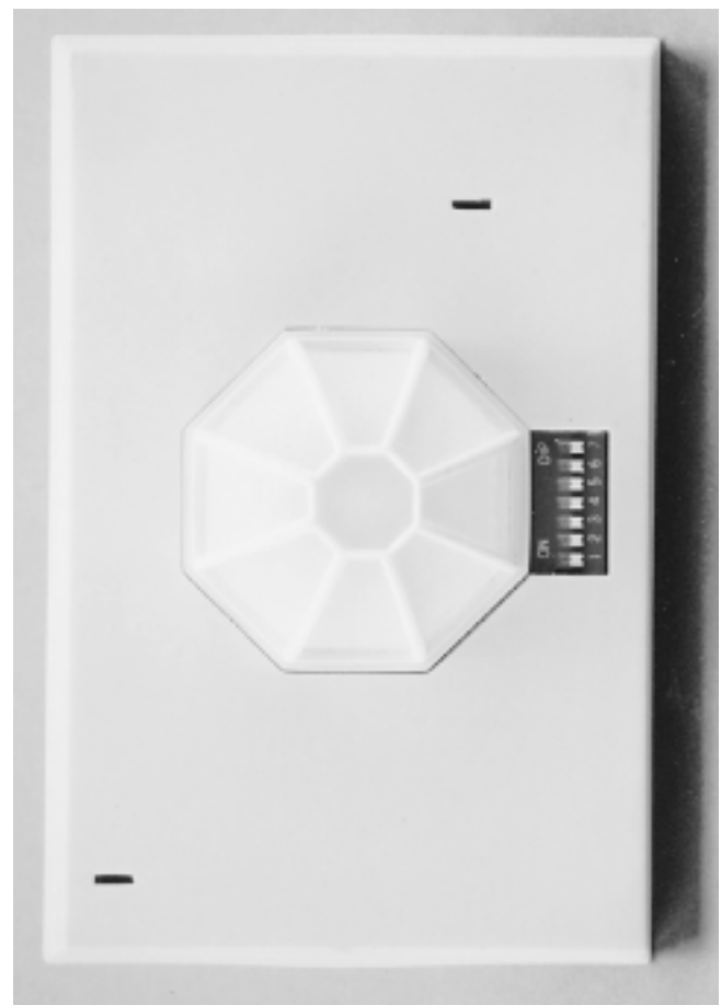
Fig. 1 Passive infrared sensor for ceiling mounting This unit sees in all directions. Installing it on the ceiling provides the most reliable coverage of the space. Settings are made with the tiny DIP switches, at the time of installation.
