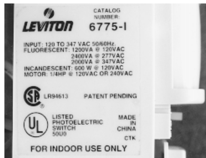
Fig. 8 Critical electrical information This infrared switch can control different kinds of electrical equipment, including motors, but the capacity ratings are different for each kind.
