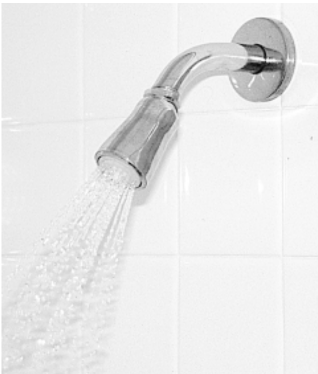
Fig. 1 Water waster This shower head has large orifices, which require a high flow rate to provide a satisfactory spray.
